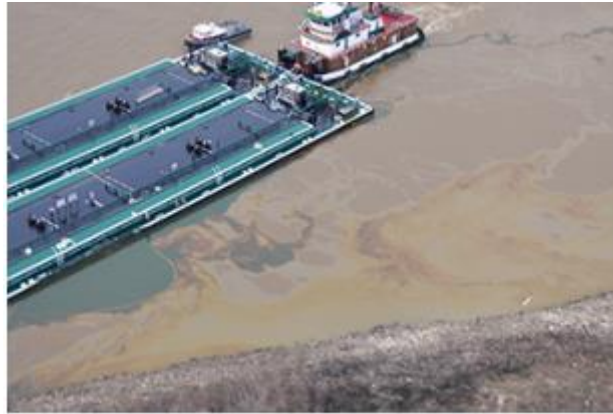
Figure 4: Leakage Caused by Barge and Towboat Collision in Lower Mississippi River [12]
