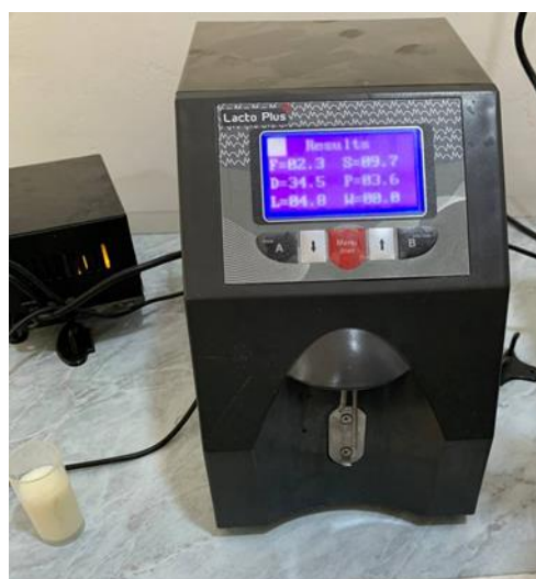
Figure 3: Lacto Plus milk analyzer showing measured parameters.
