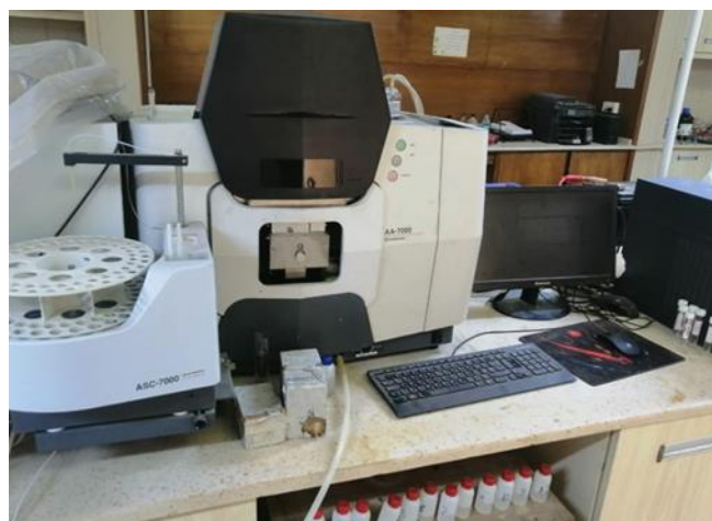
Figure 5: Atomic absorption spectrophotometer (Model AA 700 Shimadzu AAS) used in this study for determination of heavy metals.
