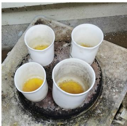
Figure 3: Digestion of cheese samples on hot plate.
