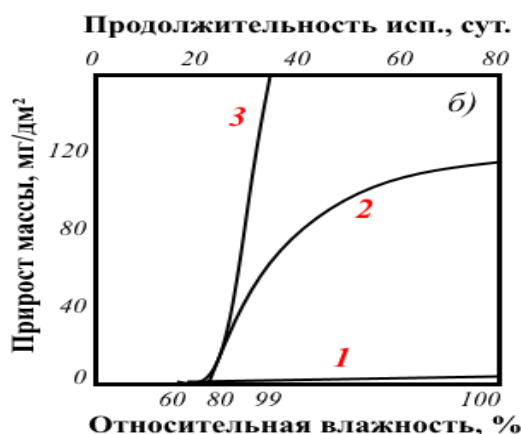
b) influence of relative humidity and atmospheric pollution on corrosion: 1 – clean air; 2 – air with 0.1% \text{SO}_2 ; 3 – air with 0.01% \text{SO}_2 and charcoal dust [4].
